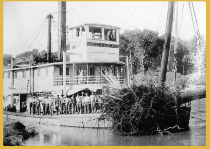
A snag boat at work on the Sacramento River, keeping the river clear of obstacles for safe shipping. (Orland Historical Society)
